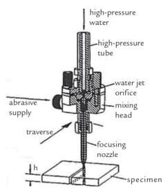
• Stand-off distance, (x): the distance between the nozzle and the impact material surface is defined as stand-off distance. As the axial and radial pressure shape of the water jet changes with its propagation, the stand-off distance parameter has significant importance about the performance process.
